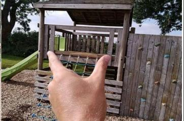
**Finding:** The platform provides access to a steep play element via a barrier with a width exceeding 1200mm and this fails to meet the requirements of BS EN1176 Part 1.
