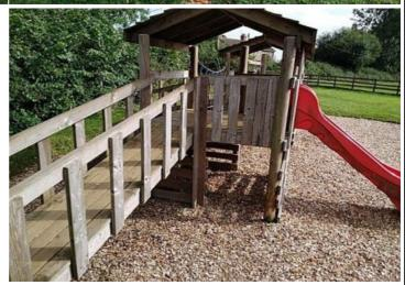
**Finding:** The unit is easily accessible and should have the appropriate barriers installed to meet the requirements of BS EN 1176 Part 1 as the height of the unit exceeds 600mm
