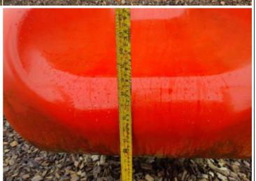
**Finding:** The height of the slide runout is in excess of 200mm and does not meet the requirements of BS EN 1176 Part 3
