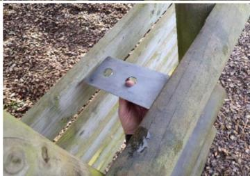
**Finding:** The item fails to meet the requirements of BS EN Action: Monitor - No remedial work recommended 1176 Part 1 4.2.7.2 for head and neck entrapment in the framework
