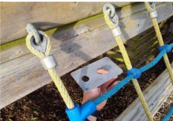
**Finding:** The item fails to meet the requirements of BS EN **Action:** Monitor - No remedial work recommended 1176 Part 1 4.2.7.2 for head and neck entrapment in between the rope net and framework
