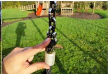
**Action:** Monitor for any further deterioration and replace when 40% worn
